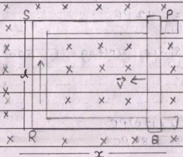
Let at any instant rod PQ covers an area PQRS. Hence rod is moving then magnetic flux linked with rod at instant of time will be
